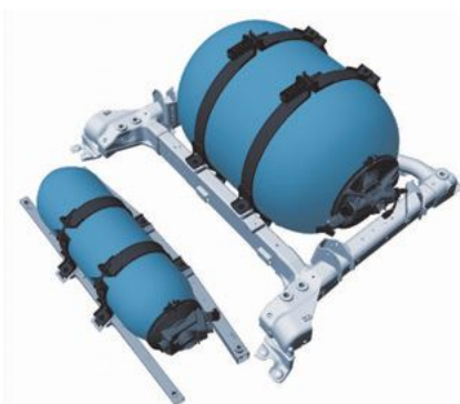
Fig. 12 Image of H 2 tank installation
