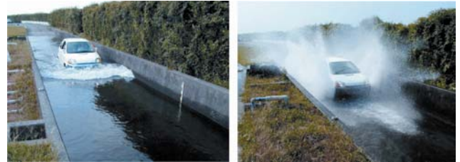
Fig. 9 Flood water test
